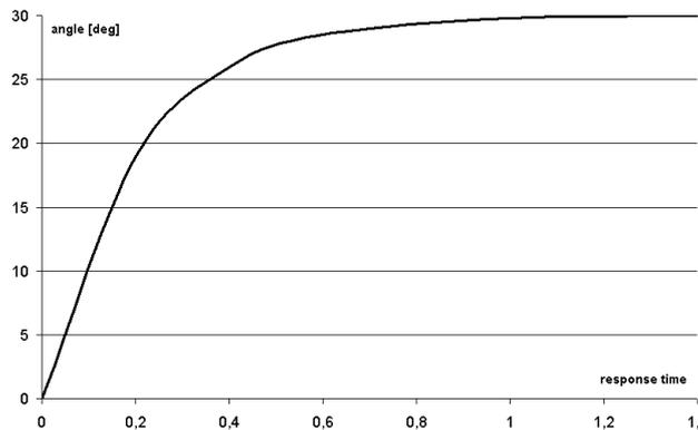
Figure 11 - Step response in time domain with 550 samples filter
