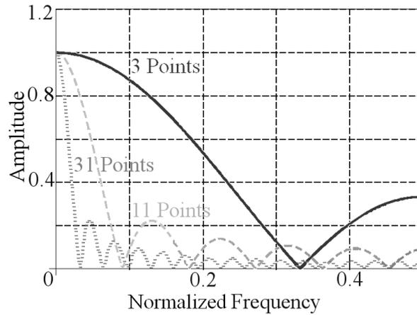
Figure 8 - Software filter response in frequency domain
