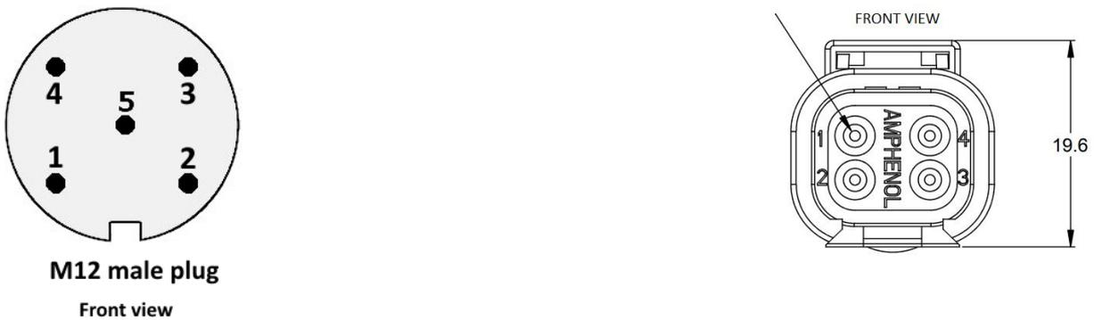
Figure 2 – OIAC3 standard M12 5 poles connector and Amphenol ATM04-4P
