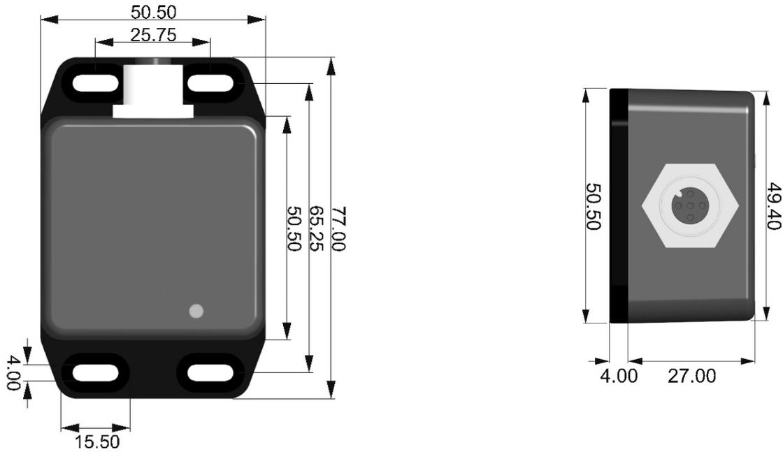
Figure 1 - OIAC3 mechanical dimensions
