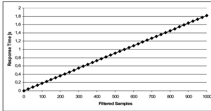
Figure 10 - Response time vs filtered samples
