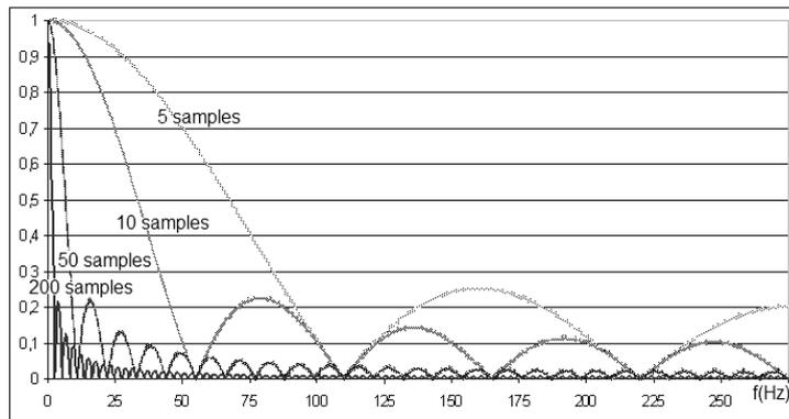
Figure 9 - Filter frequency response with different numbers of filtered samples
