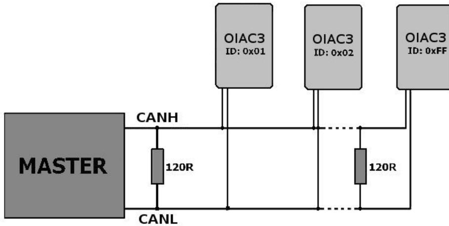
Figure 3 - OIAC3 wiring scheme
