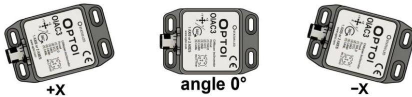
1 AXIS ZERO POSITION AND DIRECTION
