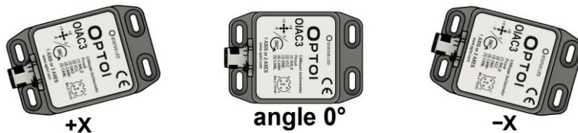
1 AXIS ZERO POSITION AND DIRECTION
